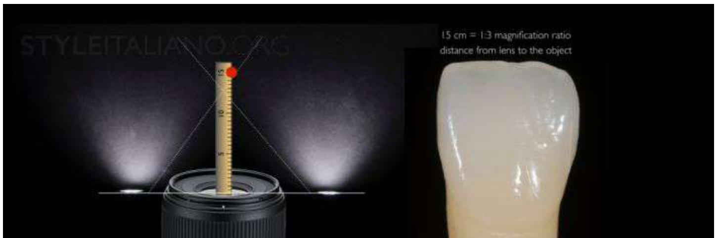
Img. 5 - Using the Nikon R1 flash directly on the lens (placed on the ring) the light is intersecting around 13 cm from the lens. At 1:3 magnification ratio the effect is as when using a ring flash.
